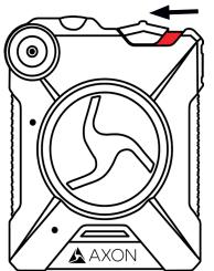
With the camera turned on, the Axon system is in the BUFFERING mode. When BUFFERING begins:
