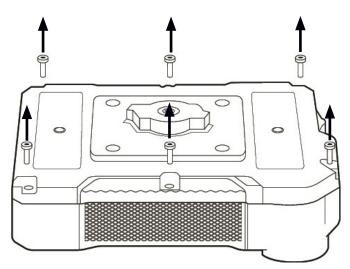
3 Remove the back of the camera.
